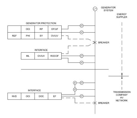
Figure 3: Typical Protection Arrangements for MV Connected Generating Plant
