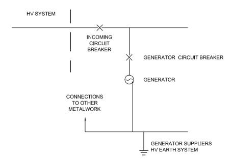
Figure 4: Typical Earthing Arrangement for MV Generator Configured for Parallel Operation (network MV earth not shown)
